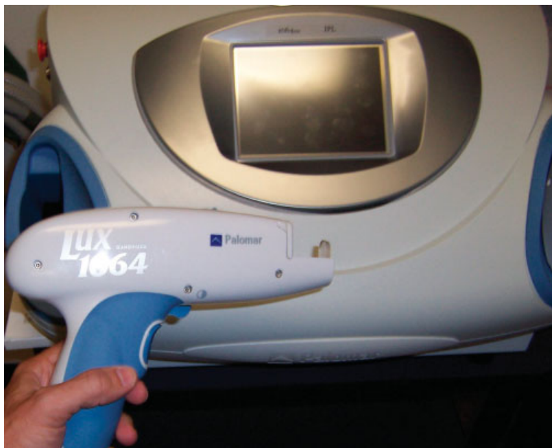
Fig. 13. Nd:YAG handpiece extending off IPL platform; handpiece houses rod and lamps.
